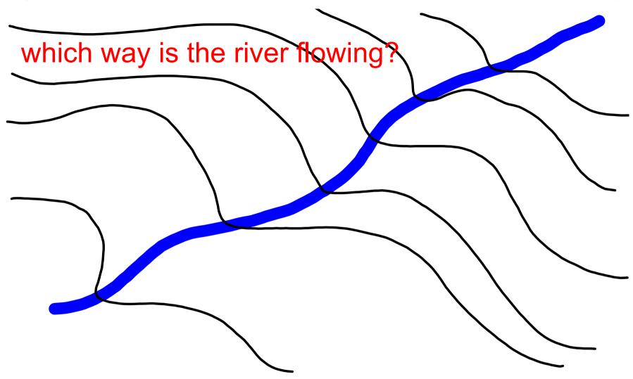
This relationship between contour lines and stream valleys is referred to as the RULE of V's. Because a V will always point upstream, the orientation of V's can always be used to determine the direction of the slope of the surface as well as the direction of the flow of the water.
