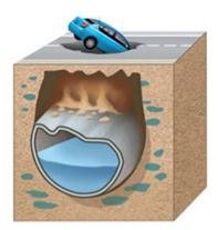
4. If sediments are very loose, a funnel-shaped sinkhole can occur quickly. But if there is a solid layer of material such as asphalt or concrete on the surface, the cavity below can remain concealed even as it grows. Once the weight becomes too much to bear, the cover collapses, and a more dangerous cylindrical sinkhole is formed.
