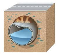
2. The loose earth fills the space created by the collapsed pipe and, in some cases, water from the pipe permeates the ground around it, weakening the surrounding soil.
