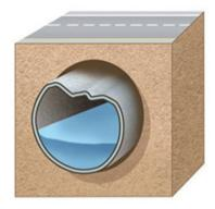
1. Infrastructure such as sewer pipes or water mains, located below loose deposits of earth, collapse as a result of erosion or age.
