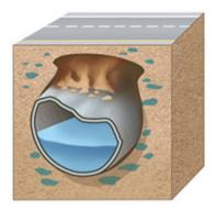
3. A cavity remains above the collapse, and expands upward to the surface.
